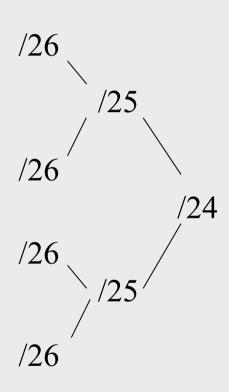
Inversely, if two networks can be "joined" together under the same netmask, which encompasses both networks, then we are *supernetting*.
