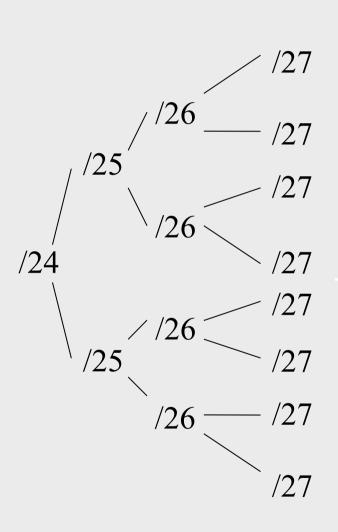
By adding one bit to the netmask, we subdivide the network into two smaller networks. This is *subnetting*.
