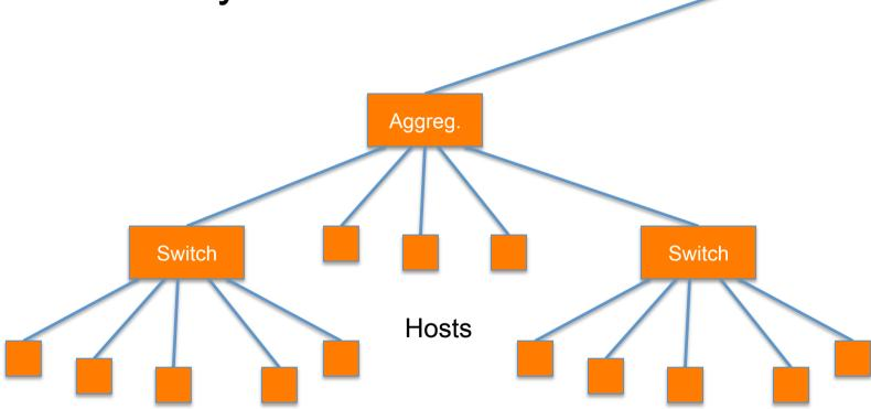
At this point, you can also add a redundant aggregation switch
