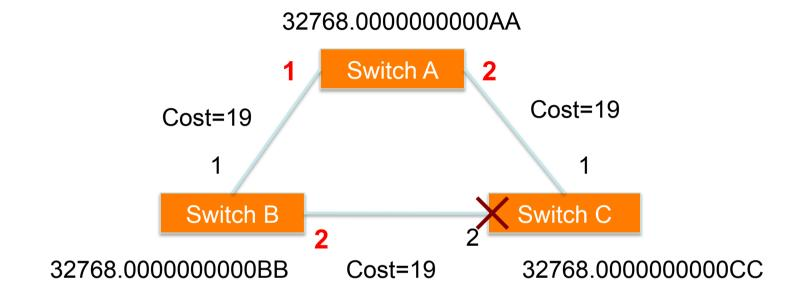
Port 2 in Switch C is then put into the Blocking State because it is neither a Root Port nor a Designated Port
