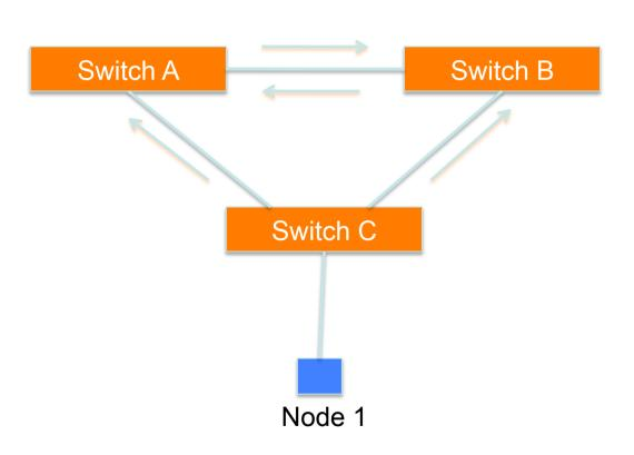
Switches A, B and C broadcast node 1's frame out every port
