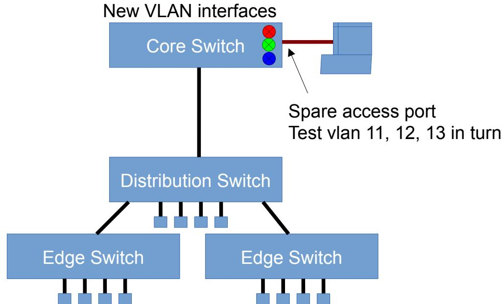
Test all client functionality, e.g. DHCP, routing
