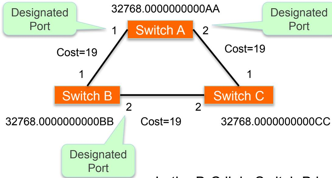
In the B-C link, Switch B has the lowest Bridge ID, so port 2 in Switch B is the Designated Port
